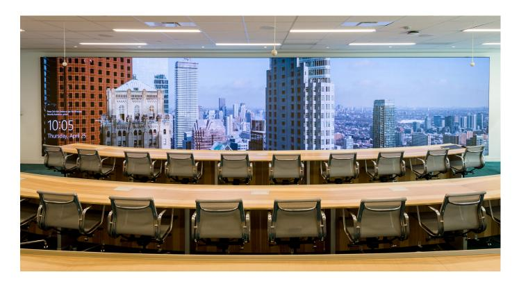
At the center of this focus is a 30-foot-long, 9-foot-high Planar® DirectLight® X LED Video Wall System in a 20x7 configuration that is installed in the auditorium of the Toronto headquarters.
