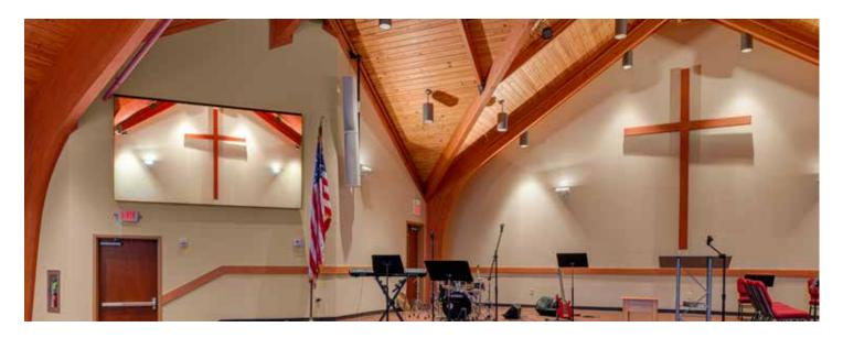
With the help of AV system designer Strategic Connections, the decision was made to integrate two 10-footlong, 5.5-foot-high Planar® TVF Series LED video walls with a 1.8mm pixel pitch (TVF1.8) in 5x5 configurations from Planar.
