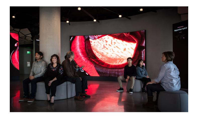
The 18-foot-long, 10-foot high LED video wall and the LED columns (11 total, each 3-foot-long and 10-foot high) are composed of Planar® CarbonLight™ CLA Series video wall displays with 1.5mm pixel pitches (CLA1.5) from .
